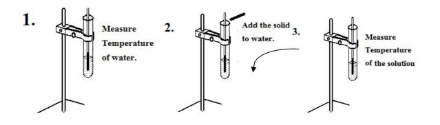
Q1. Describe an experiment to show that  $KNO_3$  dissolves in water endothermically.
