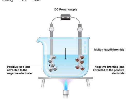
The lead ions, being positively charged, are attracted to the negative electrode.
