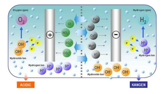
When an electric current is passed through the electrolyte, the positive ions move to the negative electrode (cathode) and the negative ions move to the positive electrode (anode).
