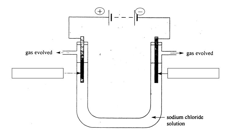
(a) The electrodes are made of graphite. Label the <u>type of electrodes</u> on the diagram above. `[1]
