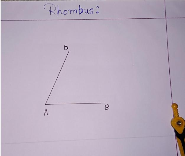
2. Measure the length of the line segment AB with the help of compass. Then place the pointer of the pencil- compass on D and draw an arc.
