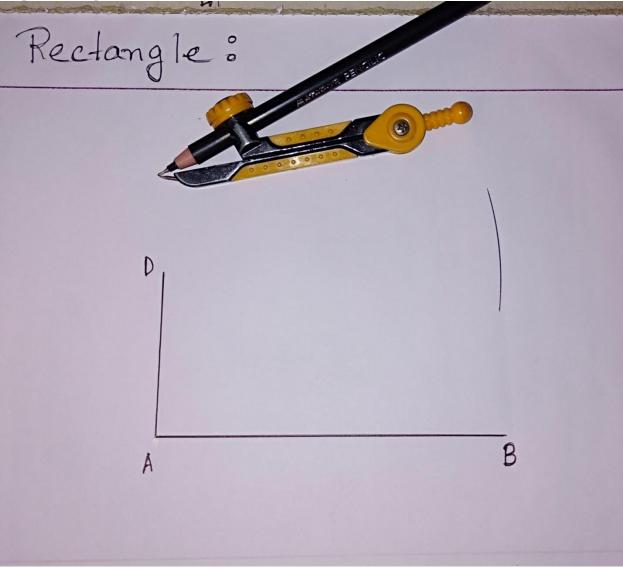
4. Similar way, measure the length of the line segment AD and draw another arc from B. Two arcs cut at the point C.
