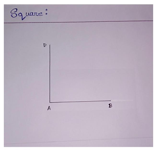
3. Measure the length of the line segment AB with the help of compass. Then place the pointer of the pencil- compass on D and draw an arc.
